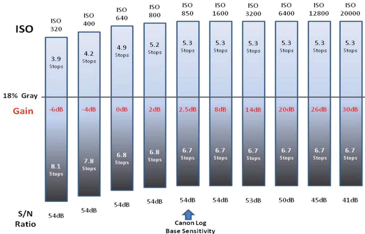
**Figure 3** Showing the overall sensitometric behavior of the EOS C300 camera. This allows assessment of the exposure latitude behavior (with respect to the reference 18% gray) with ISO setting while correlating this with the Master Gain setting and associated Luma signal to noise performance.
