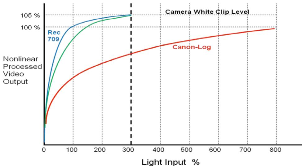
**Figure 1** *Illustrating the concept of the Canon-Log curve specifically designed to fully utilize the 800% dynamic range capability for the CMOS image sensor in order to achieve wide exposure latitude in a digital cine camera*
